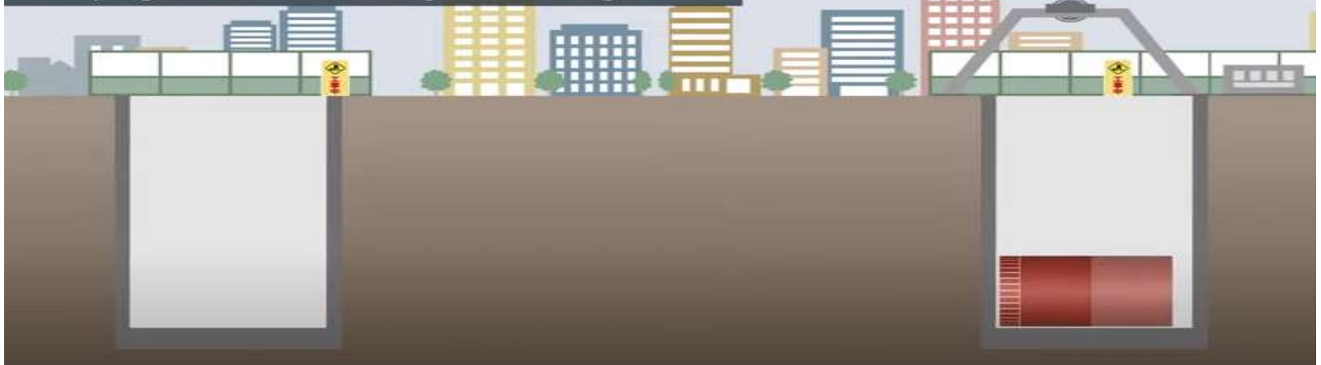
Carrying in and assembling a tunneling shield
